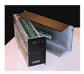
Some modules may have more or less pins, than the sockets on the matrix board. Modules must be installed that pins match at the top. Pins may not match at the bottom of a socket or module.
